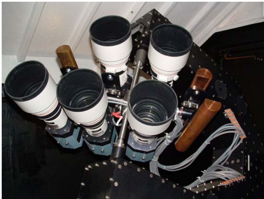
Figure. 2.11 SuperWASP observatory system with 5 cameras located at La Palma, Spain. Image credited: SuperWASP consortium.
