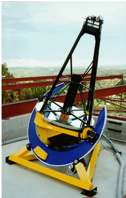
Figure 2.9 Horseshoe equatorial mount design 0.8m Cassegrain telescope at the Fairborn Observatory. Image credited: Fairborn observatory.
