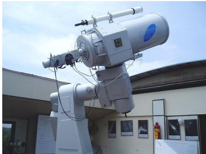
Fig. 4.1 GOTO 45cm Cassegrain Telescope
