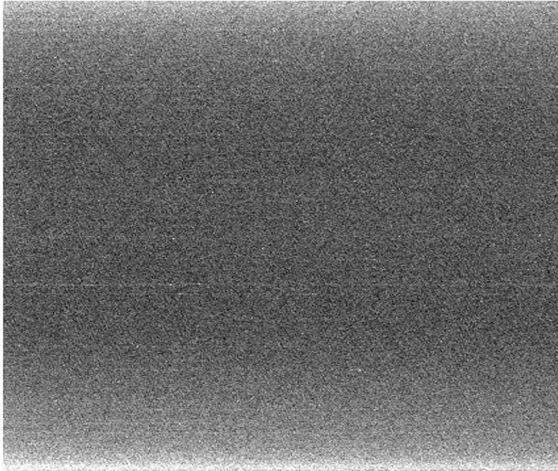
Figure 3-6 Master bias frame image used for bias noise correction of the IY UMa star. There's no any star in this image, because looking only for the noises from the instrument. And there's no any .fix exposure time.
