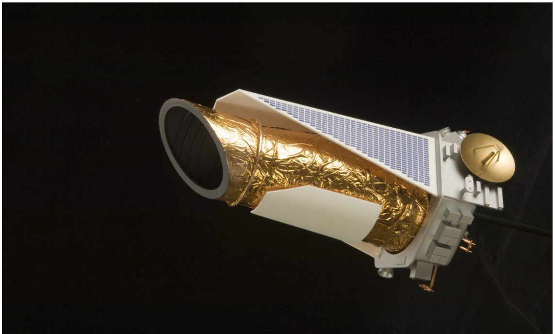
Figure 3-2 Image of the Kepler space based telescope. The cylindrical part use to collect the light of the stars. And it has solar panel system to produce the power. The main objective of the Kepler telescope is find the exoplants and extraterrestrial life.
