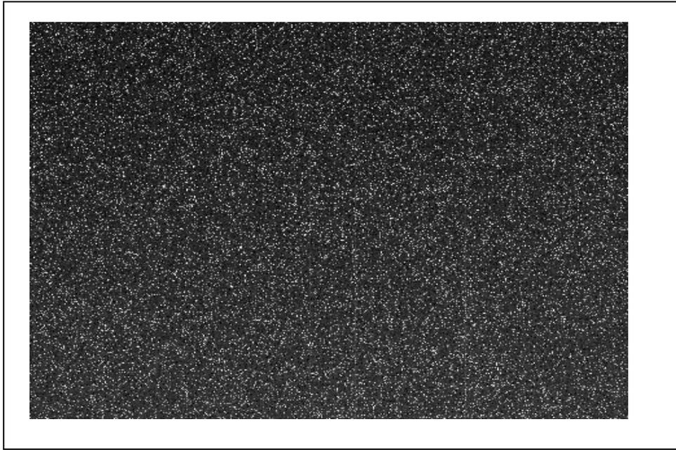
Figure 2.6 Dark Frame of the ST-7 CCD Camera
