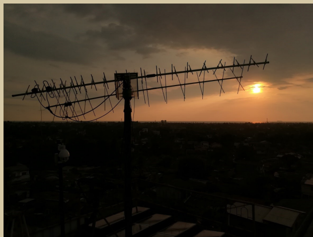
Fig.1.1 VHF/UHF Antenna with Rotation mechanism
