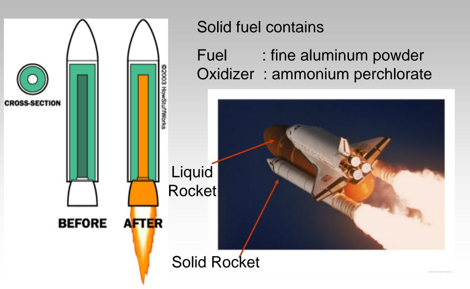
Solid-fuel rocket engines have three important advantages:
